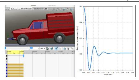
Figure 5. Computer tests execution. Suspension rod based on FSAM. Sprung weight 430 kg.
