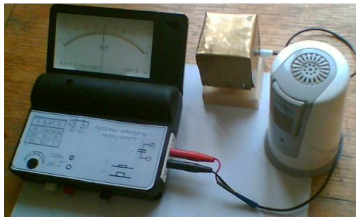
Figure 2 Appearance of the device measuring the concentration of light ions
