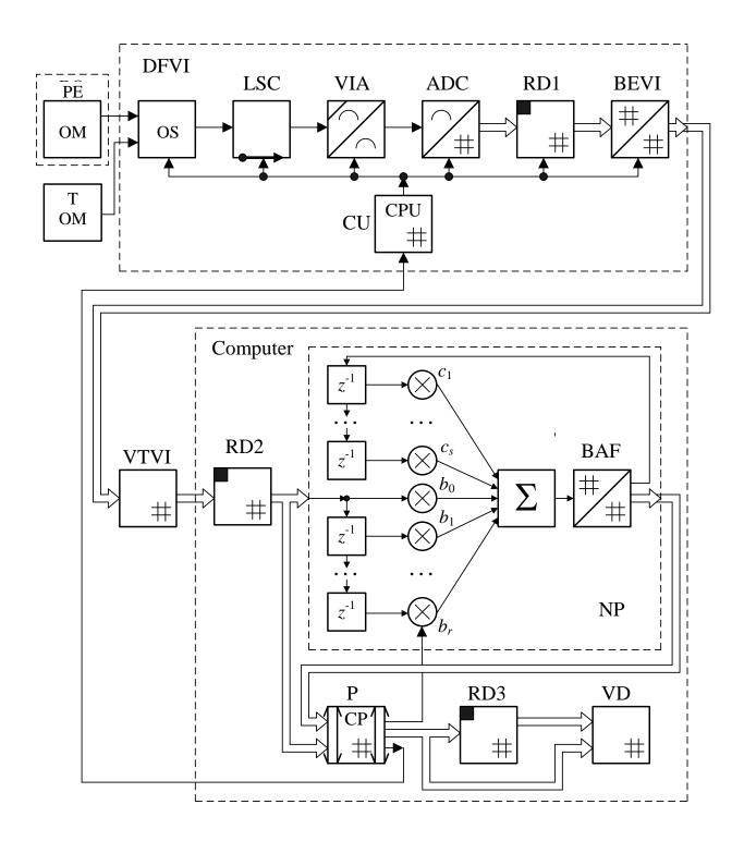
Fig. 1. Measuring system for measuring geometric parameters of objects on the basis of computerized processing of video images
