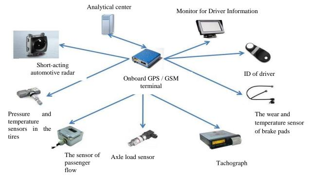
Fig. 1. Scheme of online monitoring system of wheeled passenger transport Conclusion: Designed system of monitoring allows the driver to obtain information concerning the recommended speed with maintenance of safety interval in the transport stream for the actual technical condition and the bus load and prevent malfunctions of the braking system at runtime of passenger traffic.
