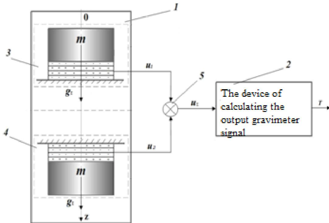
Picture 1. The block diagram of the two channel MEMS-gravimeter: 1- carcass of gravimeter, 2- device of calculating the output signal, 3- element of the first channel (mass is below), 4- element of the second channel (mass is above), 5- adder
