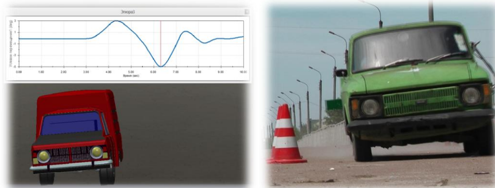
Fig. 2 The comparison of “the evasive maneuver” results in computer and road tests
