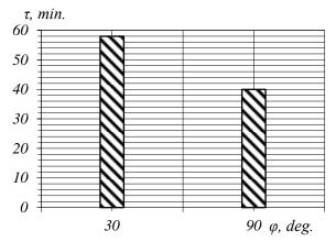
Figure 1. Dependence of  $\tau$  tool stability on its front angle in the plan  $\gamma$  at cutting speeds:
